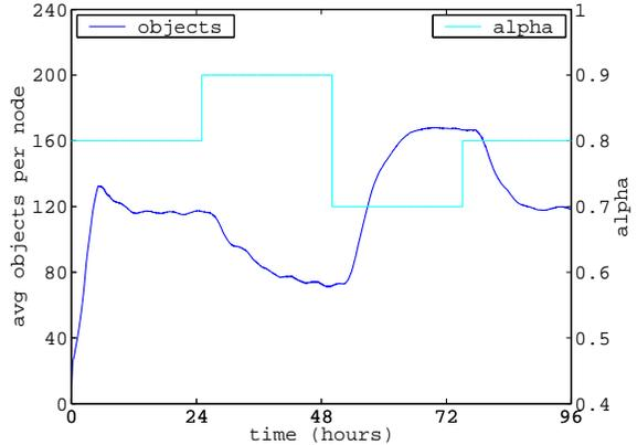
Figure 9: **Objects stored per node vs Time.** This graph shows that when the parameter of the query distribution changes, Beehive adjusts the number of replicated objects to maintain  $O(1)$  lookup performance with storage efficiency.
