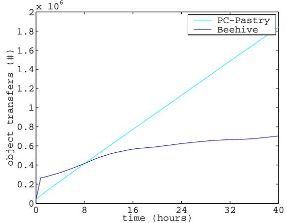
Figure 4: **Object Transfers (cumulative) vs Time.** The total amount of object transfers imposed by Beehive is significantly lower compared to caching. Passive caching incurs large costs in order to check freshness of entries in the presence of conservative timeouts.
