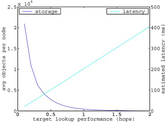
Figure 5: **Storage Requirement vs Latency.** This graph shows the average per node storage required by Beehive and the estimated latency for different target lookup performance. This graph captures the trade off between the overhead incurred by Beehive and the lookup performance achieved.
