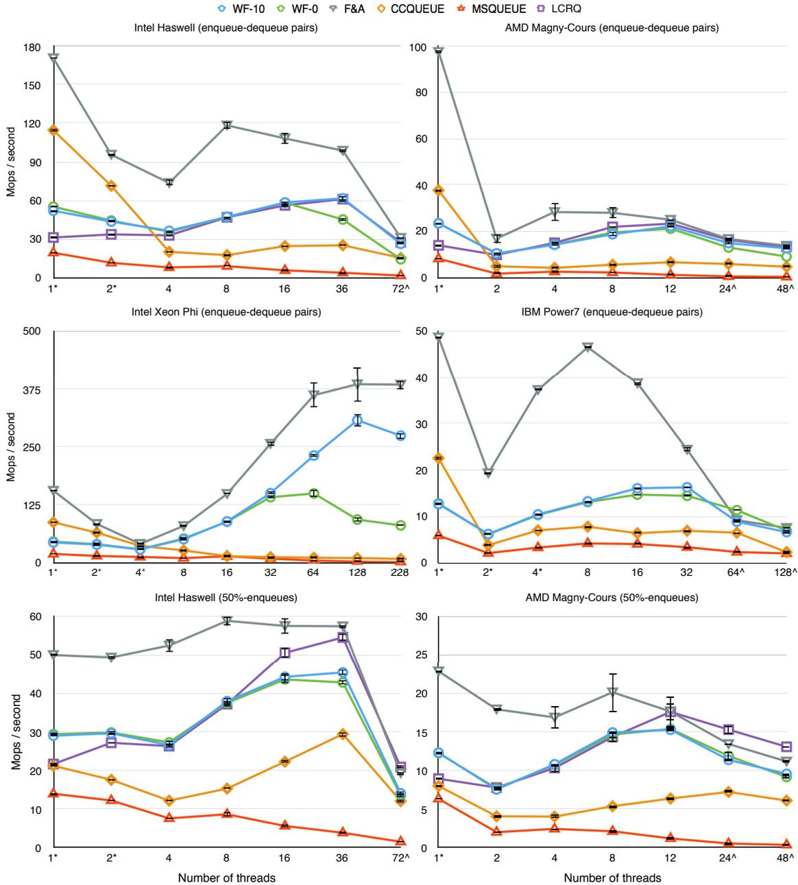
**Figure 2.** Throughput of different queues on all four platforms. There is no implementation of LCRQ for Intel Xeon Phi and IBM Power7 because the architectures lack support for CAS2. \*: executions where all threads run on the same core. ^: executions that involve multiple processors. The error bar around each data point marks the bounds for its 95% confidence interval.
