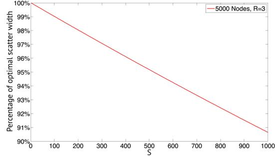
Figure 9: Comparison of the average scatter width of Copyset Replication to the optimal scatter width in a 5000-node cluster.
