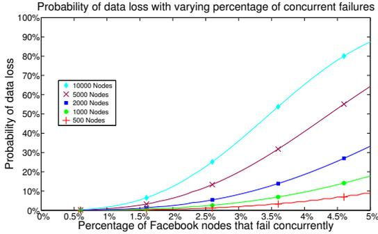
Figure 8: Data loss probability on Facebook’s HDFS cluster, with a varying percentage of the nodes failing simultaneously.
