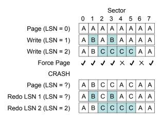
Figure 3: Torn pages and LSN-free recovery. The page is torn during the crash, but consistent once redo completes. Overwritten sectors are shaded.
