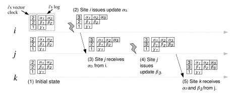
Fig. 16. Example of operation propagation using vector clocks. Symbols  $\alpha$ ,  $\beta$  and  $\gamma$  show updates submitted at *i*, *j*, and *k*, respectively. Shaded rectangles show changes at each step.
