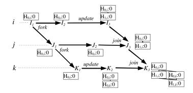
Fig. 14. Example of the use of hash histories (HHes) using the same scenario as Figure 13. The object starts as a single replica on *i* with a HH of  $H_0$ , where  $H_0$  is a hash of the current contents of the object. After an update at *i*, the HH becomes  $H_0$ - $H_1$  by appending the new contents hash. The result of merging and resolving two conflicting updates ( $K_3$ ) is represented in the HH by creating an acyclic graph as shown.
