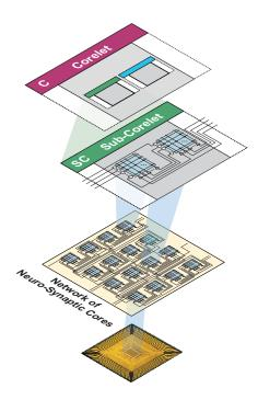
Fig. 10. A corelet is an abstraction of a TrueNorth program and is composed hierarchically from sub-corelets (other corelets) while ensuring correctness, consistency, and completeness with respect to the TrueNorth architecture.
