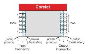
Fig. 5. A corelet is an abstraction of a network of neurosynaptic cores. The corelet has an *input* connector and an *output* connector. Each connector has a *public side* and an encapsulated *private side*. The figure also shows *pins* on each connector. On the private side, pins of the input connector connect to input axons within the network of neurosynaptic cores, and pins of the output connector connect to output neurons in the network of neurosynaptic cores.
