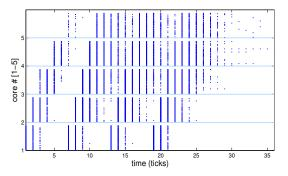
Fig. 9. A spike raster of a five-layers TrueNorth test program, with each layer composed of one seed corelet. Output spikes from the 256 neurons in each neurosynaptic core are stacked along the y-axis. Spike time is along the x-axis (1tick=1mSec).
