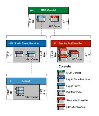
Fig. 8. A corelet diagram of the Music Composer Recognition system, provided here as a Corelet Language "Hello World" example. The application is written as a corelet class: MCR. It is hierarchically composed of two sub-corelets; a parametric Liquid State Machine (LSM) corelet and a Stackable Classifier (SC) corelet. The Corelet LSM has, in turn, two sub-corelets: Corelets Liquid and Splitter. Likewise, the Corelet SC is composed of a hierarchical classifier.
