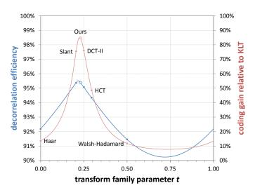
Fig. 2: Decorrelation efficiency (blue; note the vertical scale) and coding gain (red) for 21 scalar fields achieved by several transforms parameterized by  $t \in [0, 1]$ . Evidently our efficient transform is near optimal.
