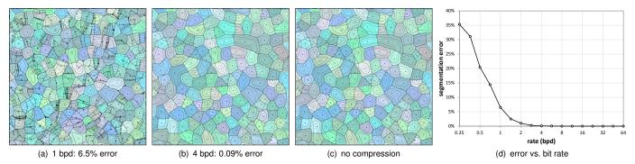
Fig. 10: (a–c) Morse segmentations of the vertical velocity field from the Rayleigh-Taylor simulation. (d) Segmentation error of unstable manifolds in terms of normalized variation of information as a function of compressed bit budget.
