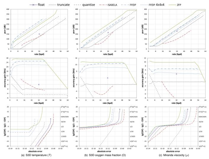
Fig. 5: Peak signal to noise ratio (top) and median accuracy gain (middle) vs. rate (bpd = bits per double) and cumulative normalized-error distribution at 32 bpd (bottom) for our ZFP method, ISABELA, original FPZIP, FPZIP applied to  $4 \times 4 \times 4$  blocks, and naïve approaches like mantissa truncation, uniform quantization, and conversion to single-precision floats. The CDFs have been transformed nonlinearly to emphasize the tails.
