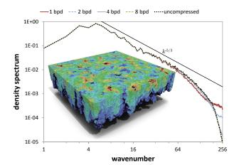
Fig. 8: Density spectrum computed over the 2D mid plane. The spectrum follows a  $k^{-5/3}$  power law in the middle region that typifies turbulent behavior. The spectrum is well represented at 4 bpd and above.
