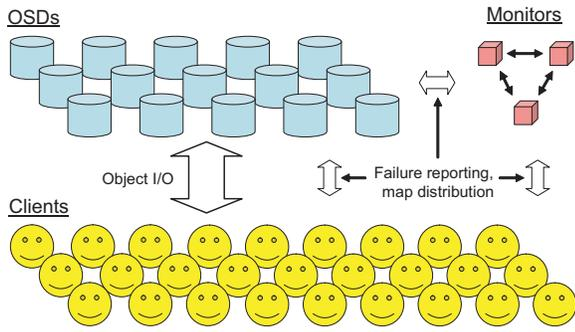
**Figure 1: A cluster of many thousands of OSDs store all objects in the system. A small, tightly coupled cluster of monitors collectively manages the cluster map that specifies cluster membership and the distribution of data. Each client exposes a simple storage interface to applications.**
