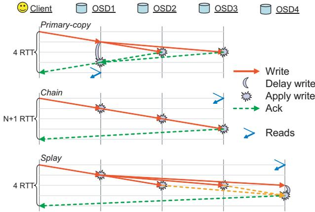
**Figure 2: Replication strategies implemented by RADOS.** Primary-copy processes both reads and writes on the first OSD and updates replicas in parallel, while chain forwards writes sequentially and processes reads at the tail. Splay replication combines parallel updates with reads at the tail to minimize update latency.
