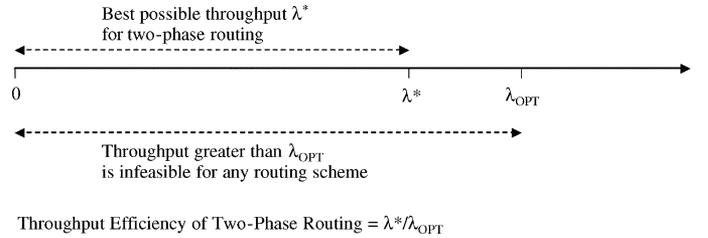
Fig. 5. Schematic illustrating throughput efficiency of two-phase routing.
