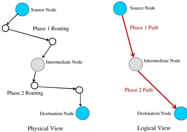
Fig. 2. Two-phase routing.
