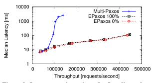
Figure 9: Latency vs. throughput for 5 replicas when batching small (16 B) commands every 5 ms.
