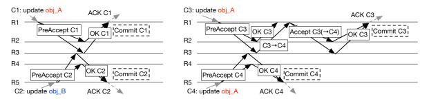
Figure 1: EPaxos message flow. R1, R2, ... R5 are the five replicas. Commands C1 and C2 (left) do not interfere, so both can commit on the fast path. C3 and C4 (right) interfere, so one (C3) will be committed on the slow path. C3  $\rightarrow$  C4 signifies that C3 acquired a dependency on C4. For clarity, we omit the async commit messages.
