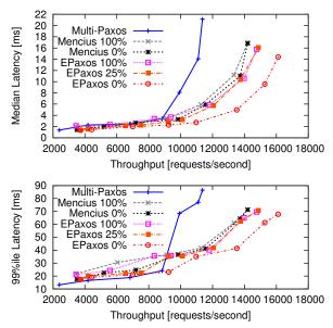
Figure 8: Latency vs. throughput for 3 replicas.
