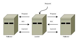
Figure 2: The protocol for message delivery. Multiple instances of this protocol can be running concurrently. The message is delivered once the leader issues the COMMIT.
