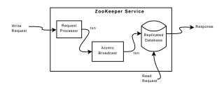
Figure 1: The logical components of the ZooKeeper service.
