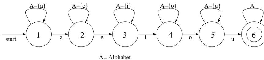
Figure 4.4: Machine to check for vowels in order
