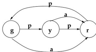
Figure 4.3: State Transitions in an Enhanced Traffic Light
