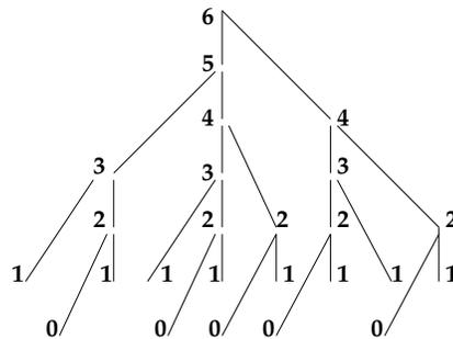
Figure 5.1: Call pattern in computing (fib 6)
