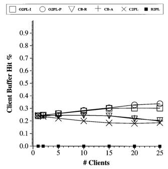
Fig. 11. Client hit rate (UNIFORM, 25% client cache, slow net).
