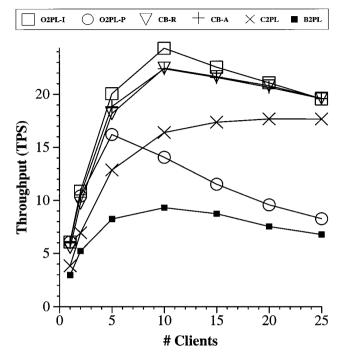
Fig. 7. Throughput (HOTCOLD, 25% client cache, slow net).
