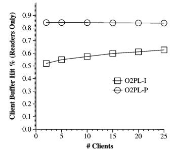
Fig. 14. Client cache hit %-readers only (FEED, 25% client cache, slow net).
