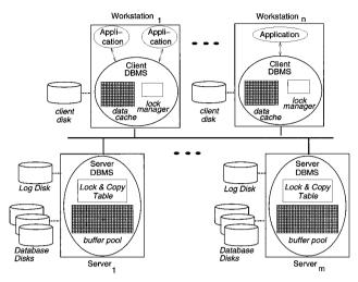
Fig. 1. Reference architecture for a data-shipping DBMS.
