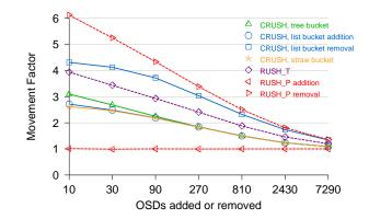
Figure 5: Efficiency of reorganization after adding or removing storage devices two levels deep into a four level, 7290 device CRUSH cluster hierarchy, versus RUSH<sub>P</sub> and RUSH<sub>T</sub>. 1 is optimal.
