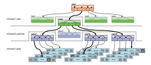
Figure 1: A partial view of a four-level cluster map hierarchy consisting of rows, cabinets, and shelves of disks. Bold lines illustrate items selected by each *select* operation in the placement rule and fictitious mapping described by Table 1.
