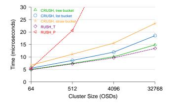
Figure 7: CRUSH and RUSH<sub>T</sub> computation times scale logarithmically relative to hierarchy size, while RUSH<sub>P</sub> scales linearly.
