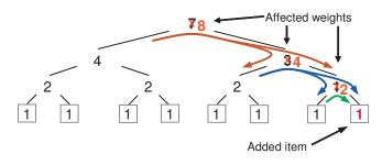
Figure 3: Data movement in a binary hierarchy due to a node addition and the subsequent weight changes.
