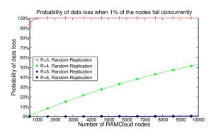
Figure 2: Simulation of the data loss probabilities of a RAMCloud cluster, varying the number of replicas per chunk.
