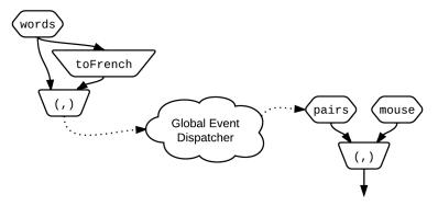
The primary subgraph – on the right – is now much smaller than the original fully-synchronous graph. It just combines two input values, a fairly quick operation. The values produced by the secondary subgraph are sent to the global event dispatcher whenever they are ready. Thus, the primary subgraph does not block mouse events while a translation is in progress. Notice that the wordPairs subgraph still ensures that translations are always paired correctly.
