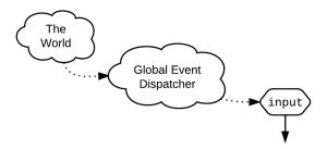
In this diagram, "The World" signifies any external data source. All interactions with the external world – mouse movements, key presses, file I/O, HTTP requests, etc. – pass from the world to the global event dispatcher.
