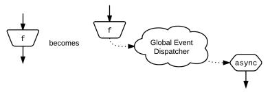
It replaces a normal graph node with an input node, allowing the computation **f** to take place while other events flow through the graph. This behavior is better explained by returning to our example.
