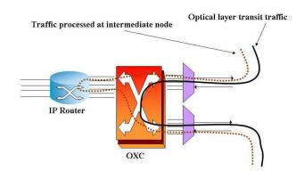
Fig. 3. Intermediate node packet processing for Two-Phase Routing in IPover-Optical networks.
